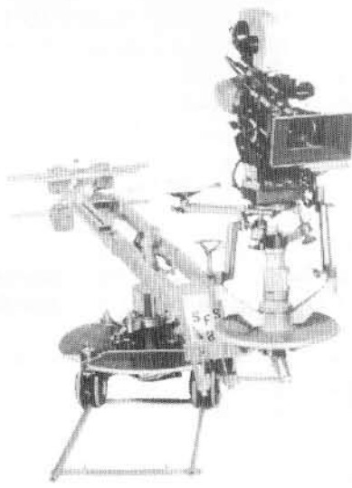
Elemack Cricket dolly, on straight track, with Jonathan Jib fitted.
