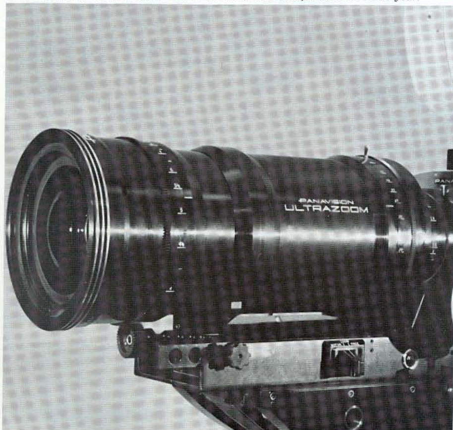
The PV Ultra Zoom. High quality 20mm-125mm with an aperture of a startling 1.9. With an anamorph it's focal length doubles to 40mm-250mm, and focus, aperture setting, and zoom can all be controlled remotely.
