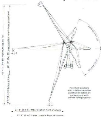
The 'Louma Crane by Samcine' is a remote control modular camera crane which is totally portable and which can make camera movements, hitherto possible only with the aid of a large truck-mounted camera crane. It has a rise and fall of over 43 ft. and a reach of 22 ft., positive pan and tilt remote controls operated by hand wheels in exactly the same manner as if the cameraman was up with the camera.
